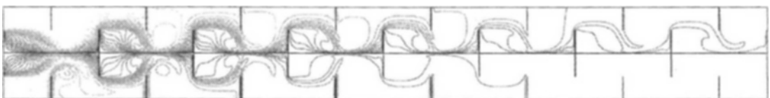
Fig. 8 Temperature contour comparison of pure convection (upper half) and combined convection and radiation (lower half)
